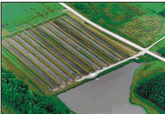
*The Flood Tolerance Laboratory at the UMC Horticulture and Agroforestry Research Center is utilized to evaluate flood tolerance of grasses, forbs and woody plants for riparian and bottomland plantings. Each channel can be independently controlled to be kept dry or flooded with flowing or standing water of different durations.*
