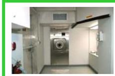
The inside door of the pass through autoclave
