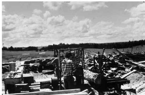
Figure 14.—Portable sawmill cutting ponderosa pine logs, Logging Camp Ranch, North Dakota. (Photo courtesy of the North Dakota Forest Service)
