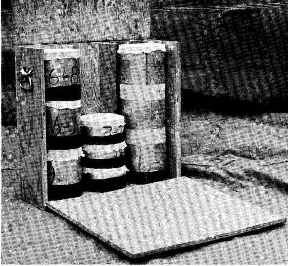
Figure 3.—Transportation-storage box containing 3-, 6-, and 18-inch samples.
