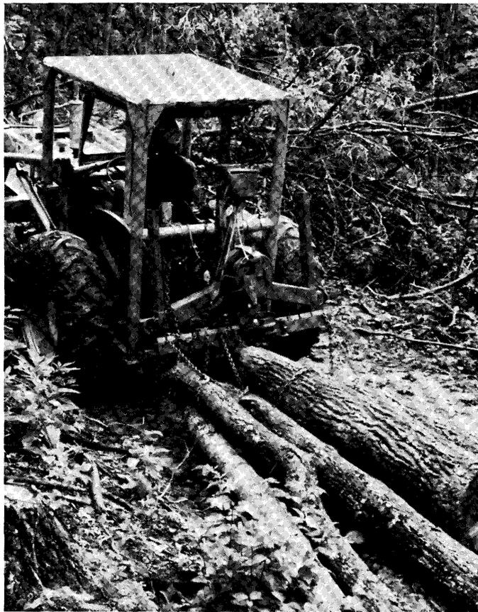
**Figure 5.—Farm tractor with rear winch used for skidding residue.**
