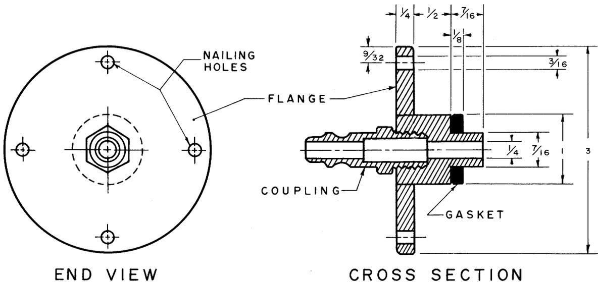
Fabrication details: A 1-inch diameter iron rod 2- $\frac{3}{16}$  inches long is turned down to  $\frac{7}{16}$ -inch diameter for  $\frac{1}{4}$  inch at one end and to  $\frac{7}{16}$ -inch diameter for  $\frac{7}{16}$  inch at the other end. A  $\frac{1}{4}$ -inch centered hole is drilled through the length of the rod and tapped for  $\frac{1}{4}$ -inch pipe threads at the  $\frac{7}{16}$ -inch end so as to accept the male part of a quick coupler.
