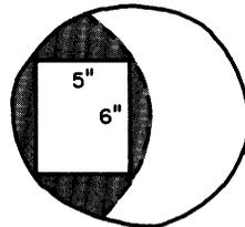
Figure 2.—Method for determining maximum retrievable timber size.
