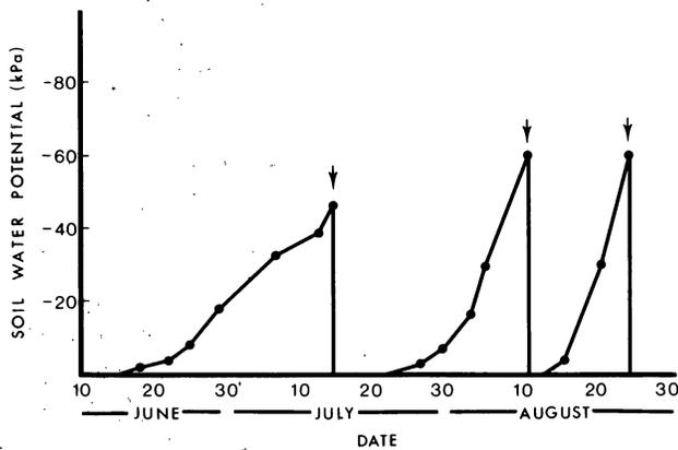
Figure 1.--Soil water potential (1kPa = 0.01 bar) determined by tensiometer for treatment 1, three cycles of stress not exceeding 60 kPa. Arrows indicate rewatering of treatment. Treatment 2 was stressed during the first cycle only and watered as was the control for the rest of the experiment. Treatment 3 received no water until August 11 and reached soil water potentials beyond the range of tensiometers.
