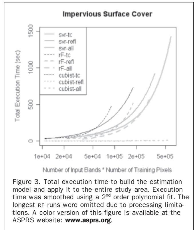
Figure 3. Total execution time to build the estimation model and apply it to the entire study area. Execution time was smoothed using a 2<sup>nd</sup> order polynomial fit. The longest RF runs were omitted due to processing limitations. A color version of this figure is available at the ASPRS website: [www.asprs.org](http://www.asprs.org).
