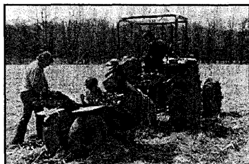
Heavy-duty tree planters and tractors are needed to cut large, deep trenches for planting hardwood seedlings.
