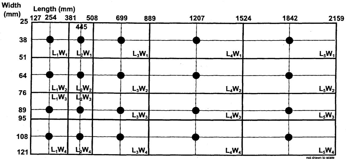
FIGURE 1. Semantic view of the 5 by 4 cutting bill space (part-group) matrix with dots indicating the part-size midpoint representing each part group.
