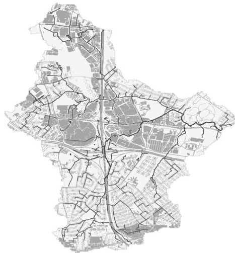
Figure 6.3. Dead Run drainage network. Dark grey lines represent open channel drainage; lighter grey lines represent the larger components of the buried storm drain system (Meierdiercks et al., 2004).
