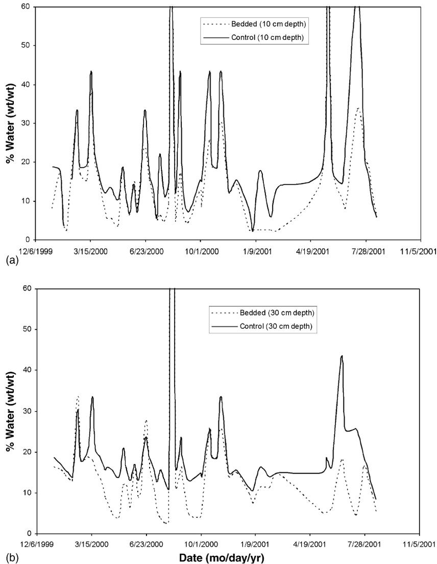
Fig. 3. Weekly gravimetric soil water content at depths of 10 cm (a) and 30 cm (b) in bedded soil and soil that was not bedded (control) at the Plowboy Bend site measured from 6 January 2000 to 17 August 2001. These readings show the wide variation in soil water content occurring between the two bedding treatments at a single location.
