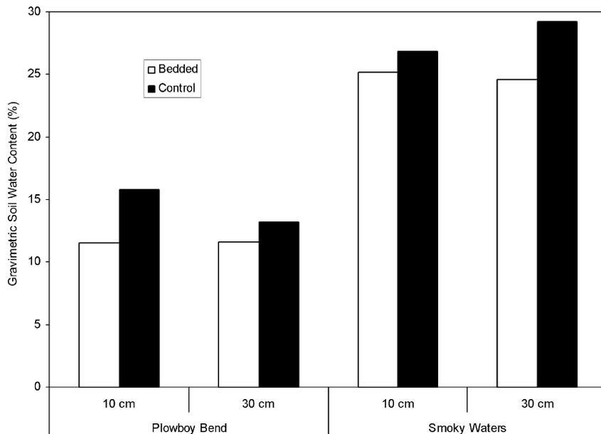
Fig. 2. Average gravimetric soil water content at 10 and 30 cm depths in bedded and non-bedded (control) soil at the two research sites. Soil water content readings were taken at four randomly selected locations per site. At each location sensors were installed at two depths each in bedded soil and in soil that was not bedded (control). Measurements were taken approximately weekly.
