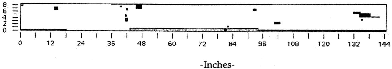
Figure 2. Sample board from Figure 1 showing only character marks included in marked areas and along edges.
