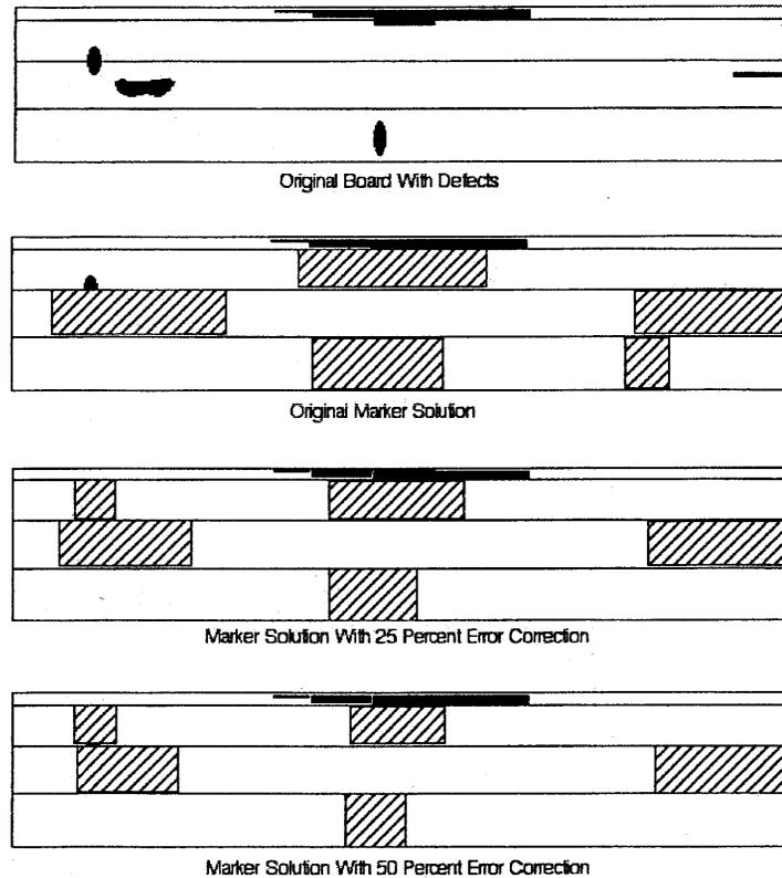
FIGURE 2: Example of board with strips showing original defect locations along with the original marker solution, a 25 percent improvement, and a 50 percent improvement.
