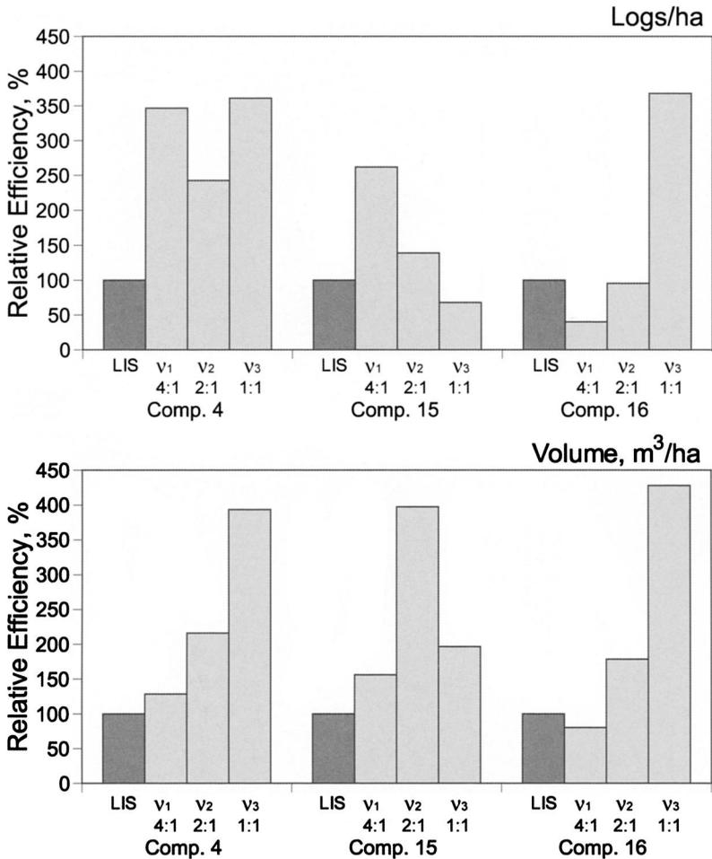
Fig. 5. Relative efficiencies of point relascope sampling inclusion angles ( $v_1$ ,  $v_2$ ,  $v_3$ ) compared to line intersect sampling (LIS) for density and volume of coarse woody material.
