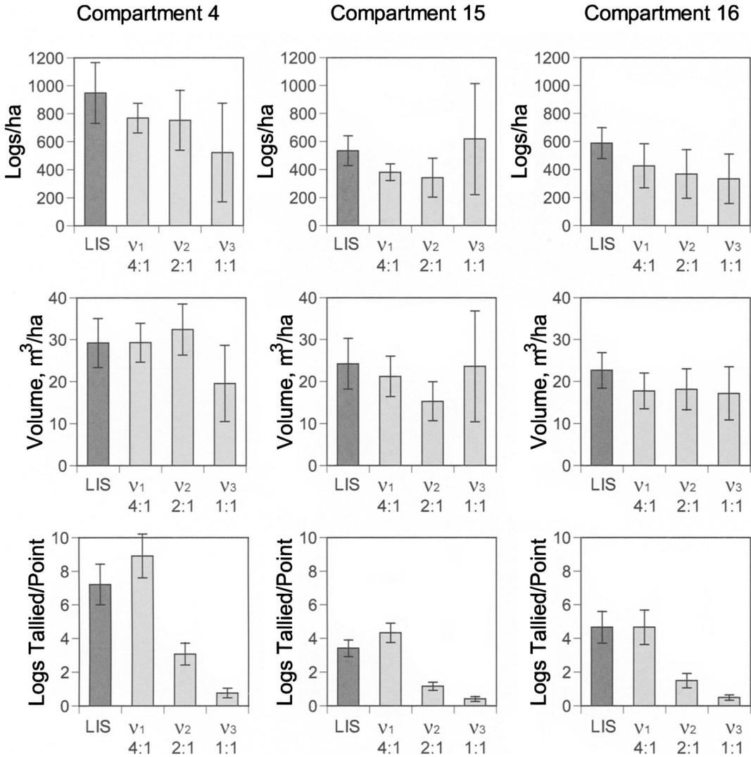
Fig. 4. Comparison of line intersect sampling (LIS) and point relascope sampling inclusion angles ( $v_1$ ,  $v_2$ ,  $v_3$ ) for all compartments with number of logs and volume/ha; in addition average number of logs tallied per point for each technique is given. Confidence intervals at the 95% level are shown about the histogram bars.
