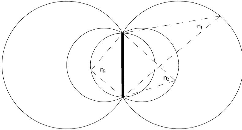
Fig. 2. Inclusion areas (partial circular regions) for point relascope sampling with three different angles (dashed lines) listed in Table 2 for a log (solid heavy line) of given length. If the sample point falls inside the inclusion area for a log, the log will be tallied with the relascope.
