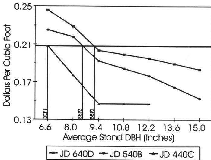
Figure 1. — Simulated delay-free skidding cost curves for JD 440C, JD 540B, and JD 640D skidders by average stand DBH; BEP1 = break-even point for JD 440C; BEP2 = break-even point for JD 540B; BEP3 = break-even point for JD 640D.
