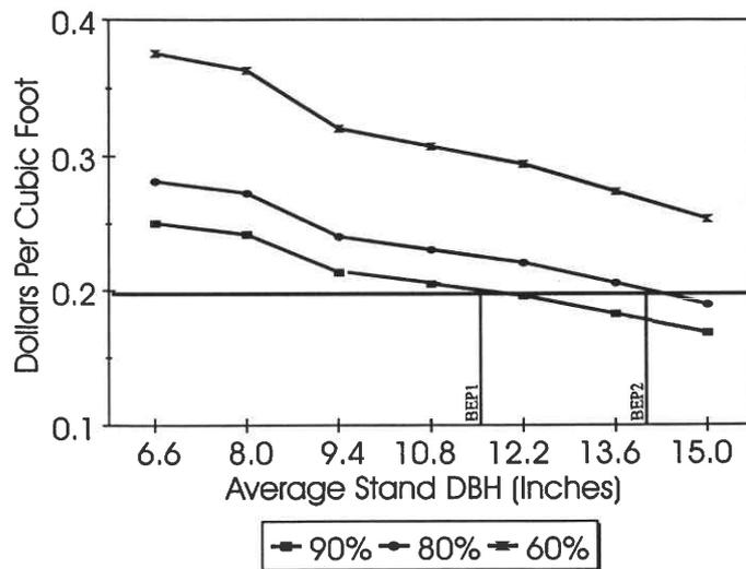
Figure 2. — Simulated skidding cost curves for JD 540B skidder at three utilization levels by average stand DBH; BEP1 = break-even point for utilization of 90 percent; BEP2 = break-even point for utilization level of 80 percent.
