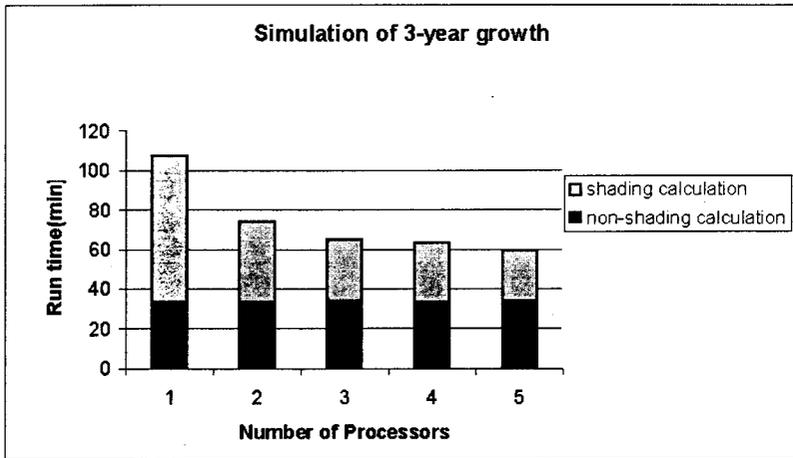
Fig. 7. Run times of three-year-old ECOPHYS tree with up to five parallel computer processors showing the high percentage of calculation time in leaf shading.
