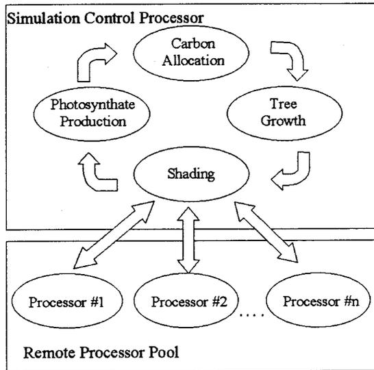
Fig. 4. Flow diagram of daily ECOPHYS cycles to the control and remote processor pool. The shade processors are dedicated to hourly shading tasks, and the control processor assists in shading, as well as in performing all other simulation activities.
