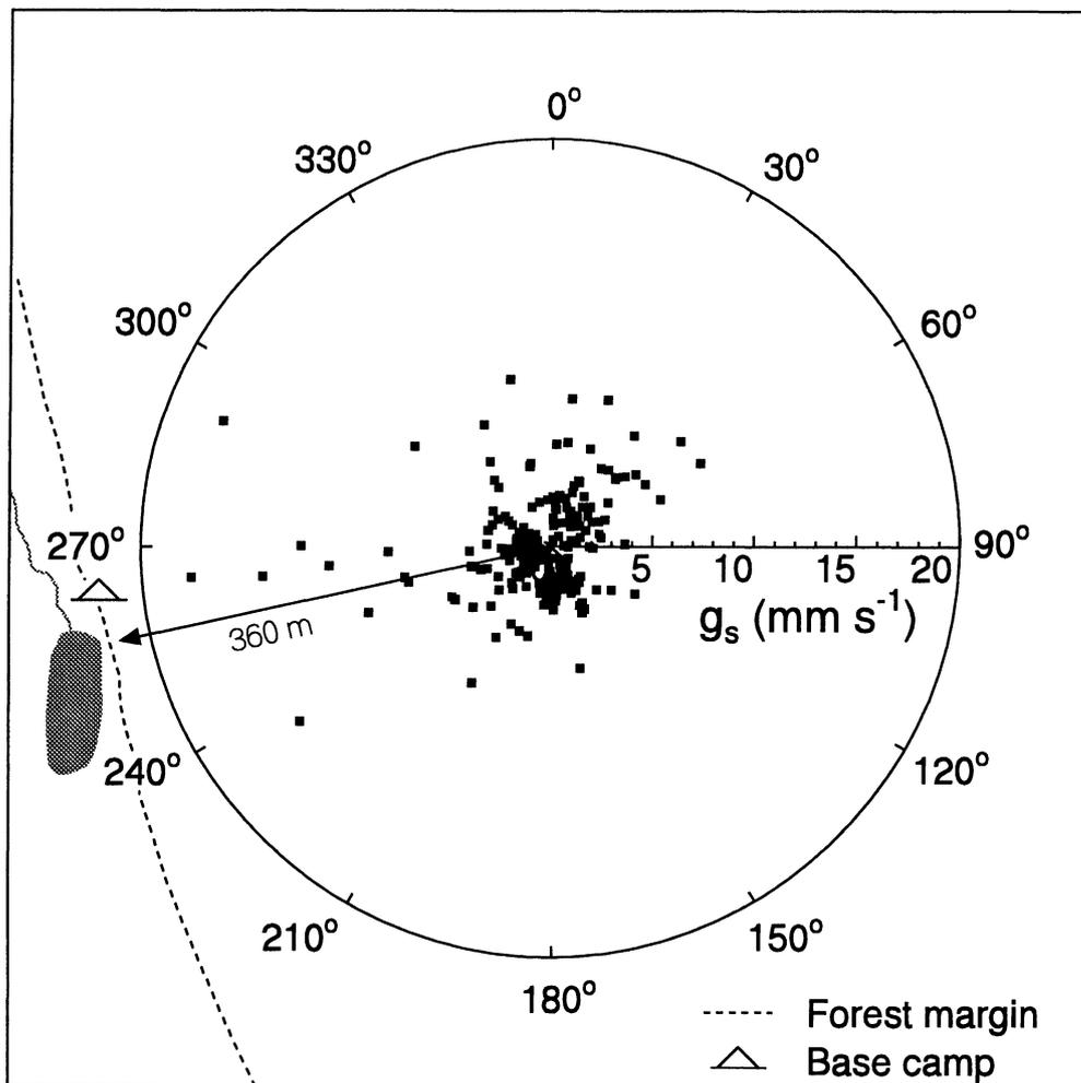
FIG. 1. Daytime surface conductance ( $g_s$ ) (13–27 August 1993) as a function of wind direction. The distance of each point from the centre indicates the magnitude of  $g_s$  and the bearing the mean wind direction during the half-hour measurement period. High values of  $g_s$  when the wind is from the west-south-west result from the presence of a small lake and marshy ground in the 'footprint' zone.
