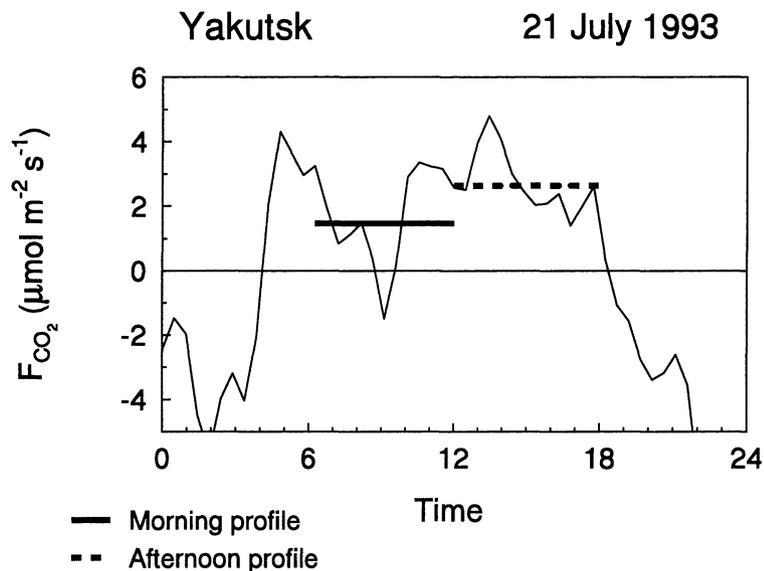
FIG. 5. Daily course of net ecosystem CO<sub>2</sub> exchange between a Siberian *Larix* forest and the atmosphere on a clear day in the middle of summer. The thin line connects smoothed, half-hourly measurements made from a tower with the eddy correlation technique. The horizontal solid and dashed bars represent mean regional CO<sub>2</sub> fluxes, estimated from aircraft measurements (see Fig. 4) using a convective boundary layer budget method, over the two time periods.
