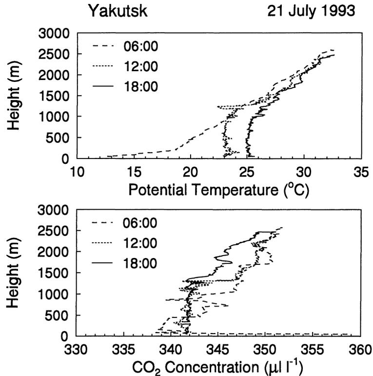
FIG. 4. Profiles of potential temperature (A) and CO<sub>2</sub> concentration (B) over *Larix* forest in eastern Siberia. During the day convective mixing minimizes gradients of these quantities in the CBL.
