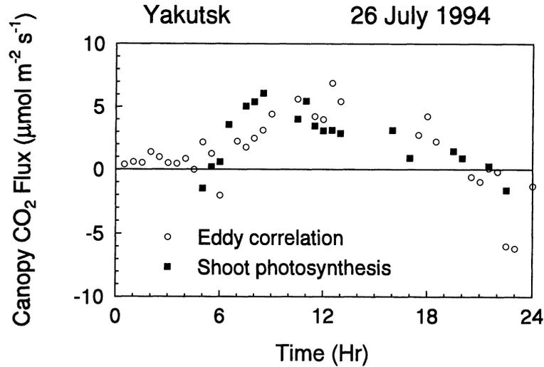
FIG. 2. Tree canopy carbon dioxide exchange rate in a Siberian *Larix* forest as the difference between fluxes measured above the forest and at 1.8 m above the forest floor (open circles) and by scaling-up leaf-level photosynthesis measurements (solid squares).
