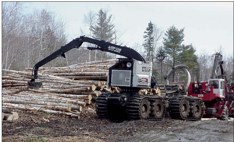
Figure 5. —Track-mounted clambunk skidder with boom attachment working on log deck (photo courtesy of Andrew Whitman, Manomet Center for Conservation Sciences).
