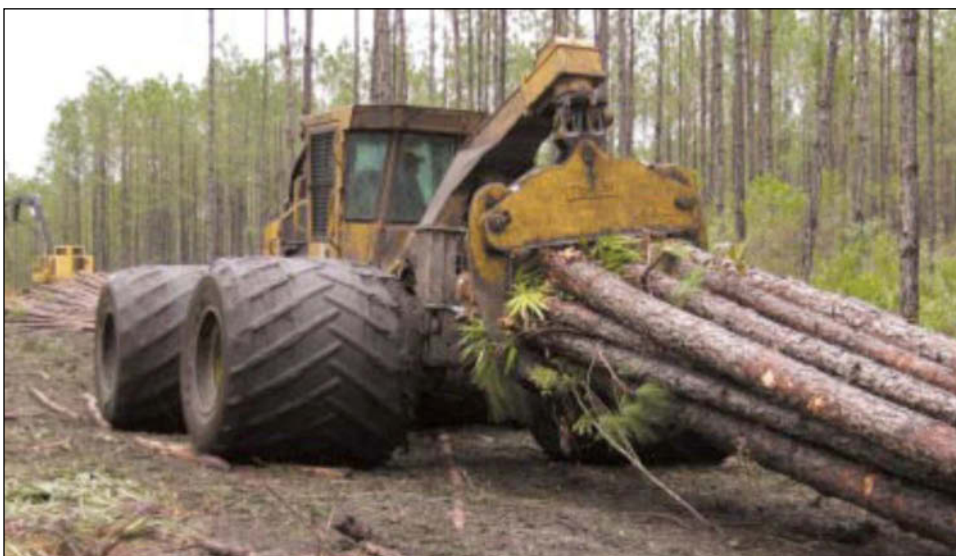
Figure 3. —Rubber-tired skidder equipped with grapple and high-flotation tires (photo courtesy of Tigercat).
