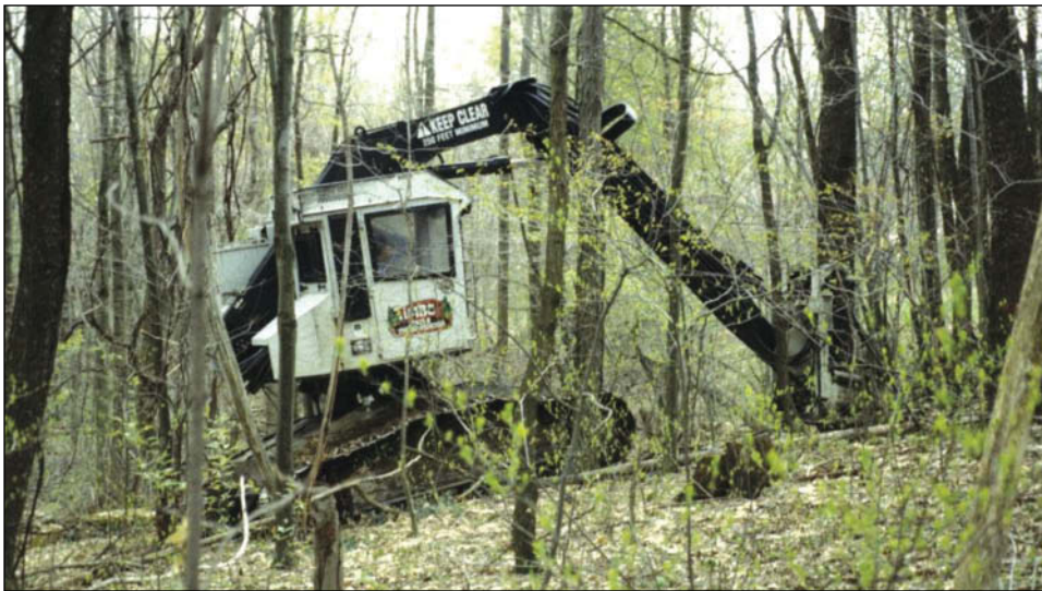
Figure 2. —Large, self-leveling, track-mounted feller buncher with accumulating felling head (photo courtesy of John Umstead, West Virginia University).
