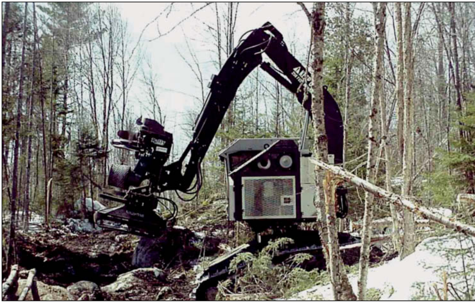
Figure 1. —Large, self-leveling track-mounted, cut-to-length processor with felling and delimiting head (photo courtesy of Andrew Whitman, Manomet Center for Conservation Sciences).
