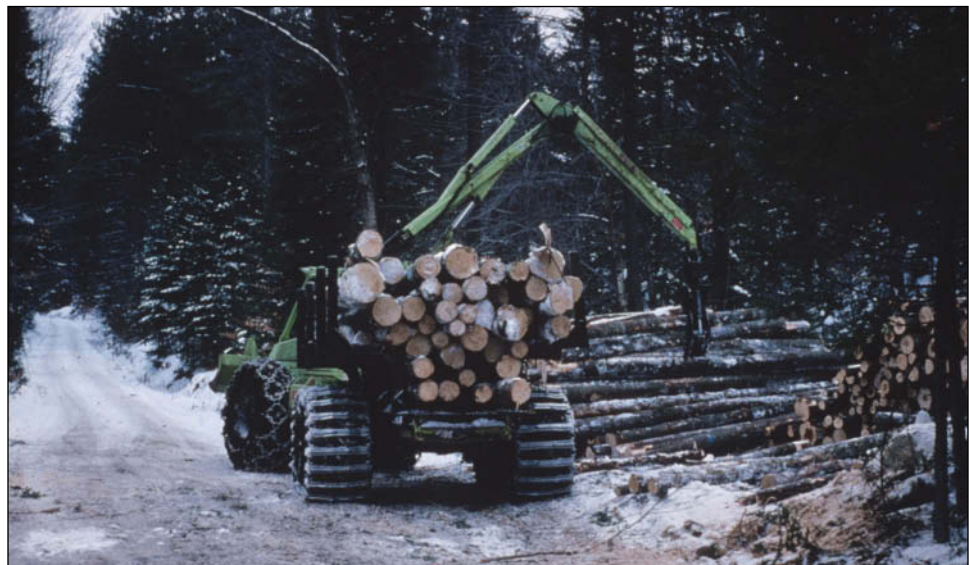
Figure 6. —Small forwarder with rubber tires and chains in the front, tracks in the rear, boom, blade in the front, unloading and sorting at the landing (photo by Neil Huyler, U.S. Forest Service, retired).
