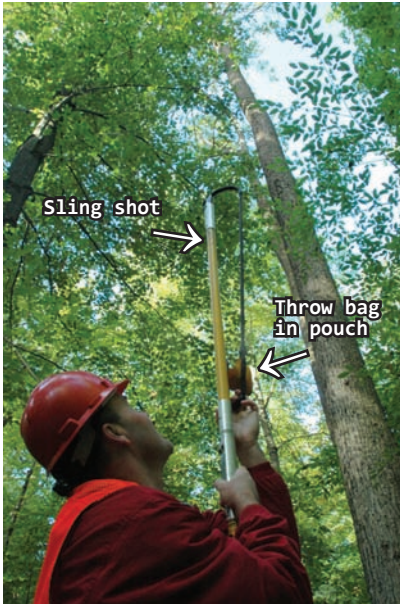
Figure 6.—Tim Fox (U.S. Forest Service) uses the Big Shot® sling shot (arrow) to shoot a throw bag (arrow) over a black ash tree branch at Fowler Woods State Nature Preserve.
