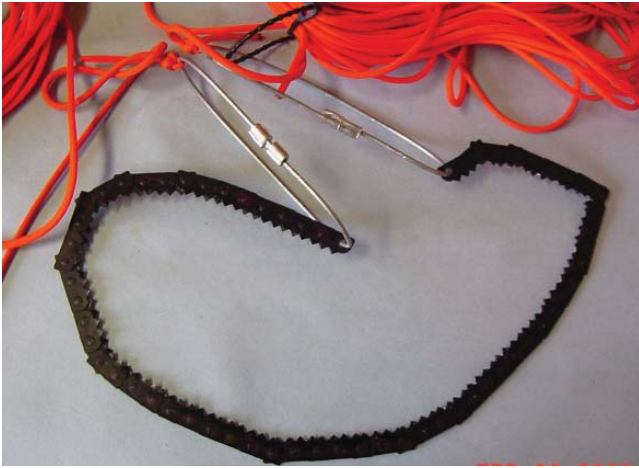
Figure 11.—Rope saw with custom attachment loops and 440 lb (200 kg) paracord.
