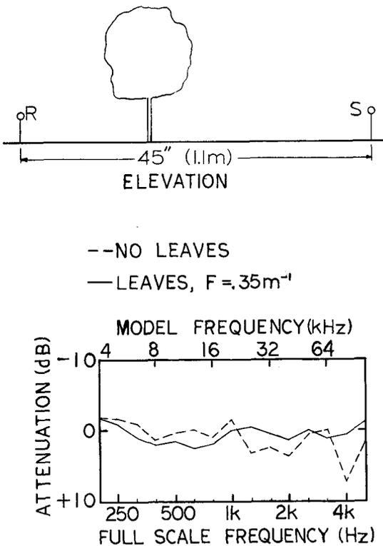
Figure 6.—Attenuation of sound by a barrier with and without trees on top.
