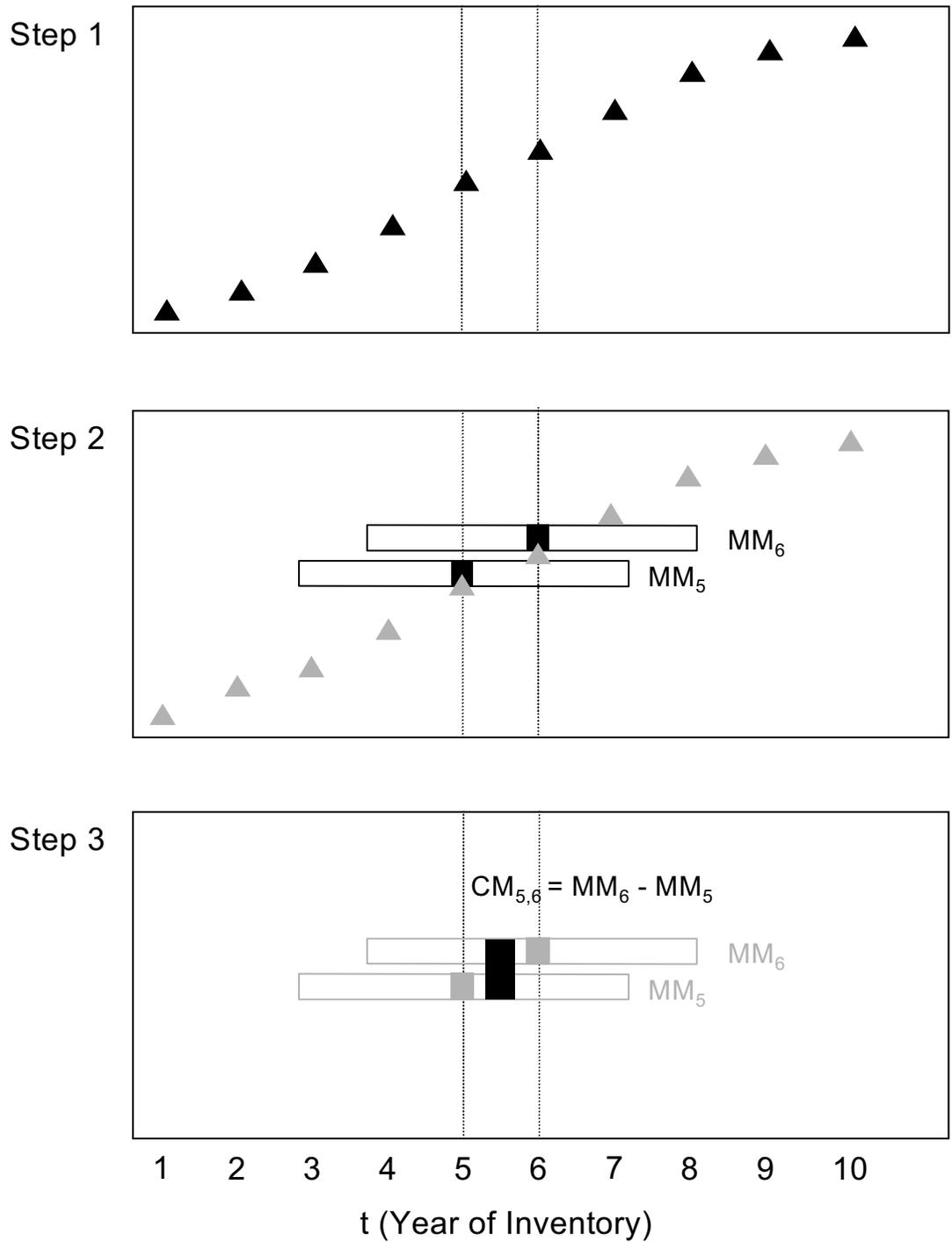
Figure 2.—Step 1 shows hypothetical means from the original data by year. Step 2 shows the years over which two moving averages were made (empty rectangle), while the dark squares represent the interpretation of the moving average as an estimator of the midpoint of the time interval. Step 3 depicts change as the difference between the two midpoint estimators.
