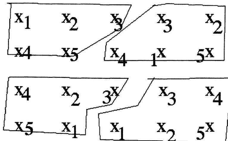
Figure 1.—A five-panel design showing four clusters of five plots each. The plot location is represented by an *x*. The panel assignment is given by the number next to the plot.
