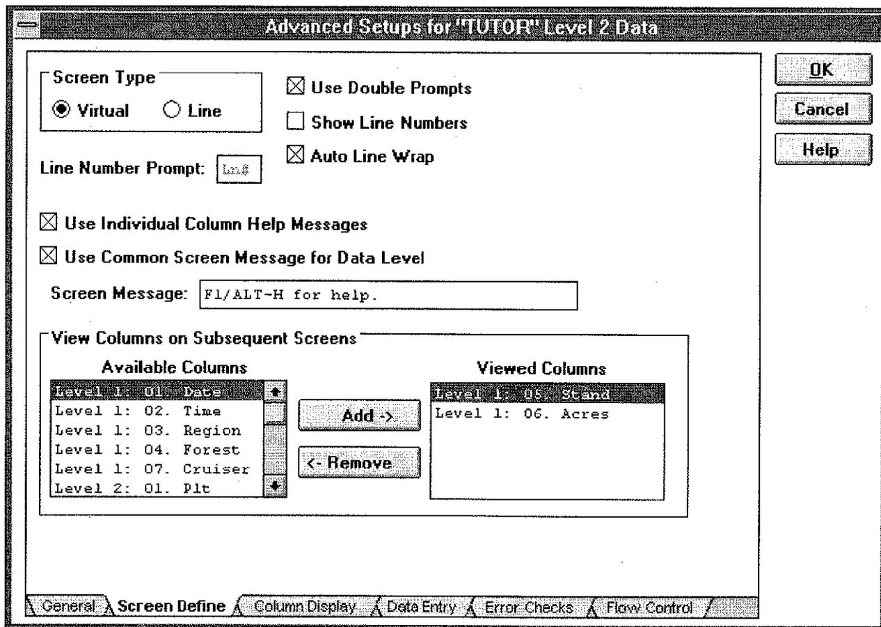
Figure 3.—Using DataPlus For DOS, Screen Define options allow specific columns from previous screens to be viewed on subsequent screens.
