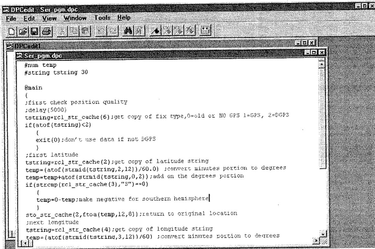
Figure 6.—With the built-in program editor in DataPlus Pro, the user can write custom programs for calculations, report printing, and data flow control.
