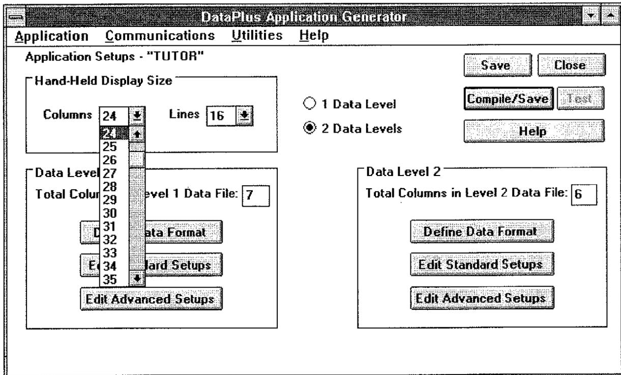
Figure 1.—DataPlus For DOS allows the application to be customized for the hand-held computer display size.
