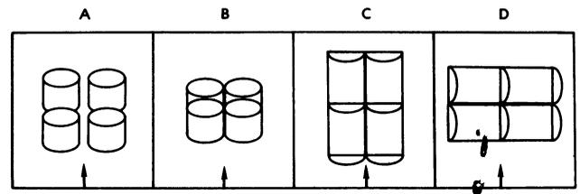
Figure 1.—Different configurations of can halves used in the four test collectors. Arrows indicate the air-flow direction. A = crosscut can halves tacked with  $\frac{1}{2}$ -inch space between cans, B = crosscut can halves tacked side-by-side in contact, C = lengthwise cut can halves tacked parallel to air flow, and D = lengthwise cut can halves tacked perpendicular to air flow.
