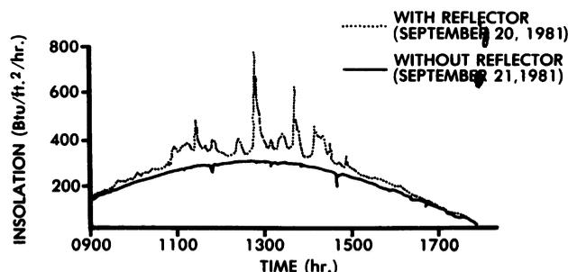
Figure 3.—Effect of reflector on useful heat collection and insolation of Collector D during two consecutive days of almost identical daily insolation.
