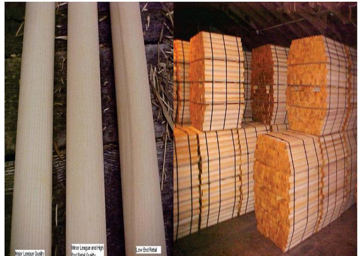
Figure 2.—Billet quality classes and grade-weight sorted bundles of finished billets awaiting shipment.
