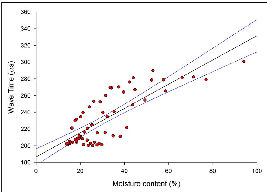
Figure 1.—Regression analysis of moisture content vs. stress wave time  $r^2 = 0.68$ , with 95 percent confidence bands.
