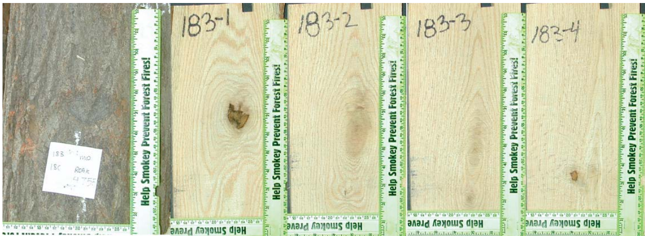
Figure 2.—Series of internal defect sections for a heavy distortion defect surface indicator.
