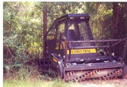
*Gyro track performs mechanical fuel reduction.*
