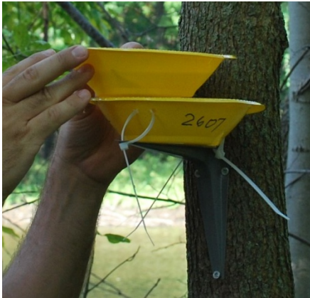
Fig. 1. Design of yellow pan trap (YPT) used for trapping EAB larval parasitoids.
