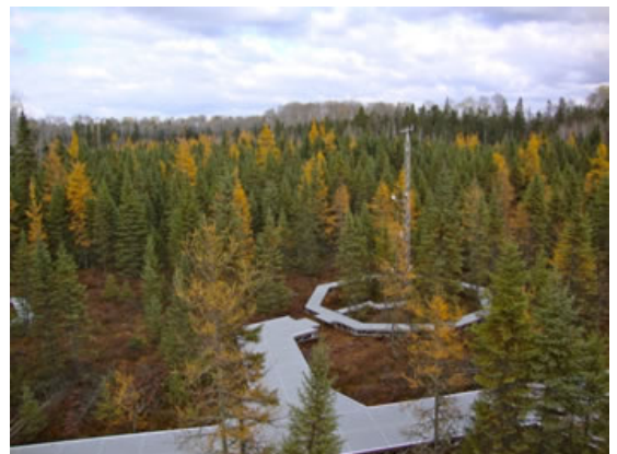
The SPRUCE Experiment consists of 10 chambers which will allow 5 temperature treatments with and without elevated carbon dioxide. Credit: USDA Forest Service
